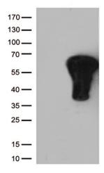
HEK293T cells were transfected with the pCMV6-ENTRY control (Left lane) or pCMV6-ENTRY FOS ([RC202597], Right lane) cDNA for 48 hrs and lysed. Equivalent amounts of cell lysates (5 ug per lane) were separated by SDS-PAGE and immunoblotted with anti-FOS (1:4000).
