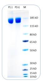
Human CD171 Protein (C-His) on SDS-PAGE under reducing condition P(+) and non-reducing condition P(-). The purity of this protein appears to be greater than 90% based on Coomassie-blue staining.
