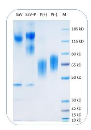
Biotinylated Human CD30 Protein (C-His-Avi) on SDS-PAGE under reducing condition P(+) and non-reducing condition P(-). The purity of this protein appears to be greater than 90% based on Coomassie-blue staining.
