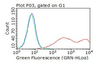
Flow cytometric analysis of living 293T cells transfected with TIGIT overexpression plasmid ([RC221447]), Red)/empty vector ([PS100001], Blue) using anti-TIGIT antibody ([TA813032]). Cells incubated with a non-specific antibody (Green) were used as isotype control (1:100).
