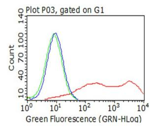
Flow cytometric analysis of living 293T cells transfected with BTLA overexpression plasmid ([RC219458]), Red)/empty vector ([PS100001], Blue) using anti-BTLA antibody ([TA812582]). Cells incubated with a non-specific antibody (Green) were used as isotype control (1:100).
