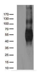
HEK293T cells were transfected with the pCMV6-ENTRY control (Left lane) or pCMV6-ENTRY CD80 ([RC206540], Right lane) cDNA for 48 hrs and lysed. Equivalent amounts of cell lysates (5 ug per lane) were separated by SDS-PAGE and immunoblotted with anti-CD80 (1:500).
