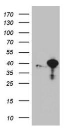
HEK293T cells were transfected with the pCMV6-ENTRY control (Left lane) or pCMV6-ENTRY RFC3 ([RC201655], Right lane) cDNA for 48 hrs and lysed. Equivalent amounts of cell lysates (5 ug per lane) were separated by SDS-PAGE and immunoblotted with anti-RFC3. Positive lysates [LY419018] (100ug) and [LC419018] (20ug) can be purchased separately from OriGene.
