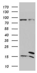
HEK293T cells were transfected with the pCMV6-ENTRY control (Left lane) or pCMV6-ENTRY SEC11A ([RC204971], Right lane) cDNA for 48 hrs and lysed. Equivalent amounts of cell lysates (5 ug per lane) were separated by SDS-PAGE and immunoblotted with anti-SEC11A (1:500). Positive lysates [LY402308] (100ug) and [LC402308] (20ug) can be purchased separately from OriGene.
