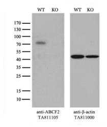
Equivalent amounts of cell lysates (10 ug per lane) of wild-type 293T cells (WT, Cat# LC810293T) and ABCF2-Knockout 293T cells (KO, Cat# [LC811907]) were separated by SDS-PAGE and immunoblotted with anti-ABCF2 monoclonal antibody [TA811105], (1:500). Then the blotted membrane was stripped and reprobed with anti-b-actin antibody ([TA811000]) as a loading control.
