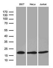
Western blot analysis of extracts (35ug) from 3 different cell lines by using anti-EDF1 monoclonal antibody (1:500).
