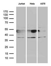
Western blot analysis of extracts (35ug) from 3 different cell lines by using anti-NFKBIE monoclonal antibody (1:500).
