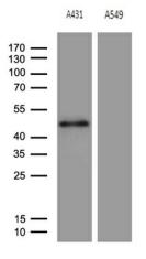
Western blot analysis of extracts (35ug) from 2 different cell lines by using anti-ELF3 monoclonal antibody (1:500).
