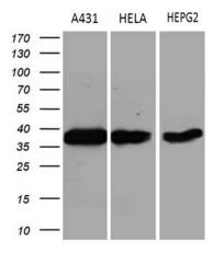
Western blot analysis of extracts (35ug) from 3different cell lines by using anti-TALDO1 monoclonal antibody? (1:500).
