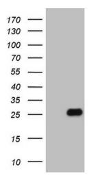
HEK293T cells were transfected with the pCMV6-ENTRY control (Left lane) or pCMV6-ENTRY FGFBP1 ([RC200819], Right lane) cDNA for 48 hrs and lysed. Equivalent amounts of cell lysates (5 ug per lane) were separated by SDS-PAGE and immunoblotted with anti-FGFBP1 (1:2000). Positive lysates [LY417486] (100ug) and [LC417486] (20ug) can be purchased separately from OriGene.
