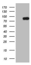
HEK293T cells were transfected with the pCMV6-ENTRY control (Left lane) or pCMV6-ENTRY CLINT1 ([RC202387], Right lane) cDNA for 48 hrs and lysed. Equivalent amounts of cell lysates (5 ug per lane) were separated by SDS-PAGE and immunoblotted with anti-CLINT1. Positive lysates [LY402360] (100ug) and [LC402360] (20ug) can be purchased separately from OriGene.
