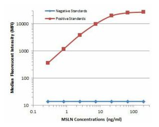
MSLN Luminex ELISA with 1A6 Capture ([TA805260]) and 3E10 Detection ([TA805261]) Antibodies. Substrate used: Recombinant Human MSLN domain expressed in E.coli.
