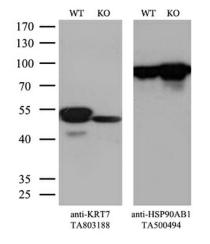
Western blot analysis of A549 cell lysate (35ug) by using anti-KRT7 monoclonal antibody. Dilution: 1:500
