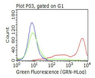
Living HEK293T cells transfected with either [RC206494] overexpress plasmid (Red), compared to an IgG isotype control, (Green) or empty vector control plasmid (Blue) were immunostained by anti-CD5 antibody ([TA801973]), and then analyzed by flow cytometry (1:100).
