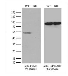
Equivalent amounts of cell lysates (10 ug per lane) of wild-type HeLa cells (WT, Cat# LC810HELA) and TYMP-Knockout HeLa cells (KO, Cat# [LC831279]) were separated by SDS-PAGE and immunoblotted with anti-TYMP monoclonal antibody [TA800961] (1:500`). Then the blotted membrane was stripped and reprobed with anti-HSP90 antibody as a loading control.
