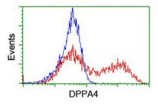
HEK293T cells transfected with either [RC205999] overexpress plasmid (Red) or empty vector control plasmid (Blue) were immunostained by anti-DPPA4 antibody ([TA800032]), and then analyzed by flow cytometry.
