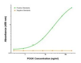
POGK Elisa with 2D5 Capture ([TA600350]) and 3D2 Detection (TA700363) Antibodies. Substrate used: Recombinant Human POGK ([TP322119])
