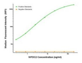
WFDC2 (HE4) Luminex Elisa with 1E12 Capture ([TA600329]) and 2A7 Detection (TA700330) Antibodies. Substrate used: Recombinant Human WFDC2 ([TP308491])
