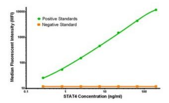
STAT4 Luminex Elisa with 2A2 Capture ([TA600183]) and 1B1 Detection (TA700192) Antibodies. Substrate used: Recombinant Human STAT4 ([TP306892])
