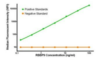
RBBP9 Luminex with 4E1 Capture ([TA600116]) and 4G3 Detection (TA700118) Antibodies. Substrate used: Recombinant Human RBBP9 ([TP302090])
