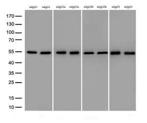
Immunoblot analysis of randomly picked 8 different lysates containing 4 different mouse IgG isotype(IgG1, IgG2a, IgG2b, IgG3) with TA592579 at 1:2000. The 8 lysates came from different sources.
