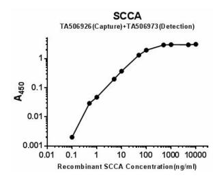
Standard curve for ELISA analysis with SCCA (SCCA1+SCCA2) recombinant protein (dilution range from 100pg/ml to 10ug/ml) using SCCA Capture Antibody (Cat# [TA506926]) at 5ug/ml and HRP conjugated SCCA Detection mAb (Cat# TA506973) at 0.025ug/ml.
