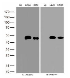
Figure A, Western blot analysis of overexpressed lysates(15ug per lane) from HEK293T cells transfected with empty plasmid ([PS100001], NC), human IDO1 plasmid ([RC206592], hIDO1), human IDO2 plasmid ([RC223337], hIDO2) using anti-IDO1 antibody [TA506372](1:500). Figure B, Western blot analysis of the same samples as figure A with anti-DDK antibody ([TA180144], 1:1000)
