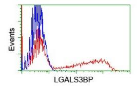
HEK293T cells transfected with either [RC204918] overexpress plasmid (Red) or empty vector control plasmid (Blue) were immunostained by anti-LGALS3BP antibody ([TA503459]), and then analyzed by flow cytometry.
