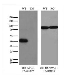
Equivalent amounts of cell lysates (10 ug per lane) of wild-type 293T cells (WT, Cat# LC810293T) and ATG3-Knockout 293T cells (KO, Cat# [LC812022]) were separated by SDS-PAGE and immunoblotted with anti-ATG3 monoclonal antibody TA503299, (1:500). Then the blotted membrane was stripped and reprobed with anti-HSP90AB1 antibody ([TA500494]) as a loading control.
