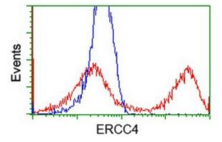
HEK293T cells transfected with either [RC223300] overexpress plasmid (Red) or empty vector control plasmid (Blue) were immunostained by anti-ERCC4 antibody ([TA503063]), and then analyzed by flow cytometry.
