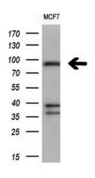
Western blot analysis of extracts (10ug) from 1 cell line by using anti-FGFR2 monoclonal antibody at 1:200.
