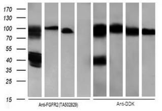
Cross-Reactivity of anti-FGFR2 ([TA502829]) with FGFR1 and FGFR3, not with FGFR4.HEK293T cells were transfected with the DDK (FLAG)-tagged DNAs of FGFR2 ([RC217098]), FGFR1 ([RC202080]), FGFR3 ([RC215533]), FGFR4 ([RC204230]) cDNA for 48 hrs and lysed. Equivalent amounts of cell lysates (5 ug per lane) were separated by SDS-PAGE and immunoblotted with anti-FGFR2 ([TA502829]). (1:500) and anti-DDK (1:2000), respectively.
