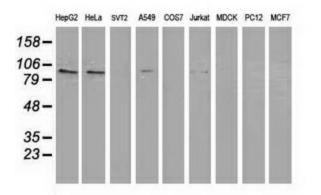
Western blot analysis of extracts (35ug) from 9 different cell lines by using anti-PRKCE monoclonal antibody.
