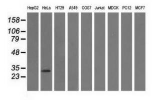
Western blot analysis of extracts (35ug) from 9 different cell lines by using anti-GSTT2 monoclonal antibody.
