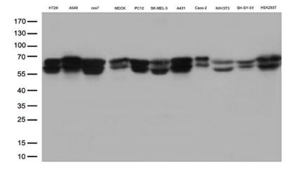
Western blot analysis of extracts (35ug) from 11 cell line lysates by using anti-IGF2BP2 monoclonal antibody (1:500).
