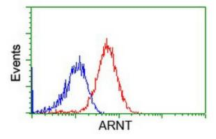
Flow cytometric Analysis of Hela cells, using anti-ARNT antibody ([TA501249]), (Red), compared to a nonspecific negative control antibody (TA50011), (Blue).
