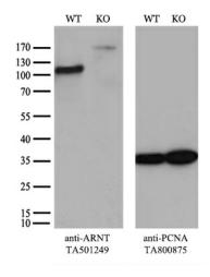
Equivalent amounts of cell lysates (10 ug per lane) of wild-type HeLa cells (WT, Cat# LC810HELA) and ARNT-Knockout HeLa cells (KO, Cat# [LC834429]) were separated by SDS-PAGE and immunoblotted with anti-ARNT monoclonal antibody [TA501249] (1:100). Then the blotted membrane was stripped and reprobed with anti-PCNA antibody as a loading control.
