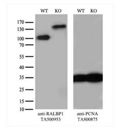
Equivalent amounts of cell lysates (10 ug per lane) of wild-type HeLa cells (WT, Cat# LC810HELA) and RALBP1-Knockout HeLa cells (KO, Cat# [LC833874]) were separated by SDS-PAGE and immunoblotted with anti-RALBP1 monoclonal antibody [TA500953] (1:500). Then the blotted membrane was stripped and reprobed with anti-PCNA antibody as a loading control.
