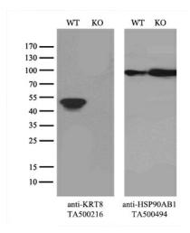
Equivalent amounts of cell lysates (10 ug per lane) of wild-type Hela cells (WT, Cat# LC810HELA) and KRT8-Knockout Hela cells (KO, Cat# [LC810123]) were separated by SDS-PAGE and immunoblotted with anti-KRT8 monoclonal antibody [TA500216], (1:1000). Then the blotted membrane was stripped and reprobed with anti-HSP90AB1 antibody ([TA500494]) as a loading control.
