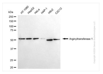
Western blotting analysis using antiarginyltransferase 1 antibody . Total cell lysates (30 µg) from various cell lines were loaded and separated by SDS-PAGE. The blot was incubated with anti-arginyltransferase 1 antibody and HRP-conjugated goat anti-rabbit secondary antibody respectively. Image was developed using anti-NaQ<sup>™</sup> ECL Substrate Kit .
