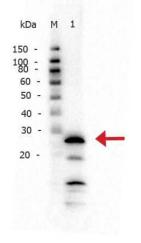
Western Blot of Rabbit anti-Trypsin antibody. Lane 1: Trypsin (Bovine). Load: 50 ng per lane. Primary antibody: Trypsin antibody at 1:1,000 overnight at 4°C. Secondary antibody: Peroxidase rabbit secondary antibody at 1:40,000 for 30 min at RT. Block: Blocking Buffer for Fluorescent Western Blotting for 30 min at RT. Predicted/Observed size: 25 kDa for Trypsin. Other band(s): Low molecular weight bands could correspond to autocatalytic fragments.
