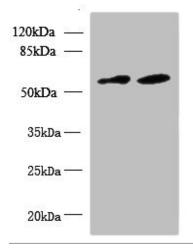
Western blot All lanes: KBTBD4 antibody at 10µg/ml Lane 1: U87 whole cell lysate Lane 2: NIH/3T3 whole cell lysate Secondary Goat polyclonal to rabbit IgG at 1/10000 dilution Predicted band size: 59, 60 kDa Observed band size: 59 kDa
