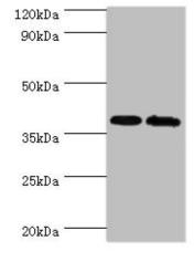
Western blot All lanes: PBK antibody at 6µg/ml Lane 1: Hela whole cell lysate Lane 2: Mouse gonad tissue Secondary Goat polyclonal to rabbit lgG at 1/10000 dilution Predicted band size: 37, 38 kDa Observed band size: 37 kDa
