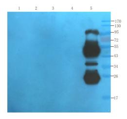
Western Blot using anti-IL2R antibody TA385810 Mouse lipocyte (lane 1), mouse spleen (lane 2), mouse thymus (lane 3), mouse lymph node (lane 4) and human thyroid tumour (lane 5) samples were resolved on a 10% SDS PAGE gel and blots probed with TA385810 at 1.5 µg/ml before being detected by a secondary antibody. The expected band size (31 kDa) is seen in the human-derived sample, as well as further bands that are specific to human.
