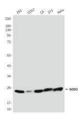
Western blot analysis of SOD2 in 293, COS7, C6, 3T3 and Hela lysates using SOD2 antibody.
