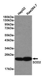
Western blot detection of SOD2 in HepG2 and Raw264.7 lysates using SOD2 Rabbit pAb (1:1000 diluted). Predicted band size: 25KDa. Observed band size:22KDa.
