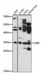
Western blot analysis of extracts of various cell lines, using USB1 antibody (TA383132) at 1:3000 dilution. | Secondary antibody: HRP Goat Anti-Rabbit IgG (H+L) at 1:10000 dilution. | Lysates/proteins: 25ug per lane. | Blocking buffer: 3% nonfat dry milk in TBST. | Detection: ECL Basic Kit. | Exposure time: 180s.
