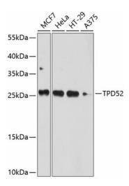
Western blot analysis of extracts of various cell lines, using TPD52 antibody ([TA382748]) at 1:1000 dilution. | Secondary antibody: HRP Goat Anti-Rabbit IgG (H+L) at 1:10000 dilution. | Lysates/proteins: 25ug per lane. | Blocking buffer: 3% nonfat dry milk in TBST. | Detection: ECL Basic Kit. | Exposure time: 10s.
