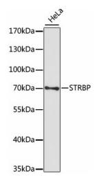
Western blot analysis of extracts of HeLa cells, using STRBP antibody (TA382153) at 1:1000 dilution. | Secondary antibody: HRP Goat Anti-Rabbit IgG (H+L) at 1:10000 dilution. | Lysates/proteins: 25ug per lane. | Blocking buffer: 3% nonfat dry milk in TBST. | Detection: ECL Basic Kit . | Exposure time: 90s.
