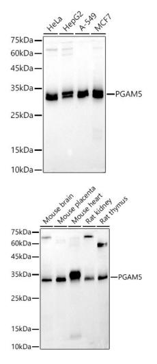
Western blot analysis of extracts of various cell lines, using PGAM5 antibody (TA379841) at 1:500 dilution. |Secondary antibody: HRP Goat Anti-Rabbit IgG (H+L) at 1:10000 dilution. |Lysates/proteins: 25ug per lane. |Blocking buffer: 3% nonfat dry milk in TBST. |Detection: ECL Basic Kit . |Exposure time: 30s.
