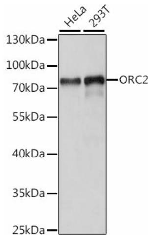
Western blot analysis of various lysates using ORC2 Rabbit pAb ([TA379494]) at 1:1000 dilution. Secondary antibody: HRP-conjugated Goat anti-Rabbit IgG (H+L) (AS014) at 1:10000 dilution. Lysates/proteins: 25µg per lane. Blocking buffer: 3% nonfat dry milk in TBST. Detection: ECL Basic Kit (RM00020). Exposure time: 10s.
