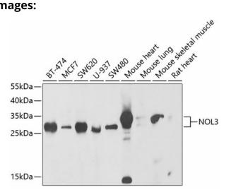
Western blot analysis of extracts of various cell lines, using NOL3 antibody (TA379203) at 1:1000 dilution. | Secondary antibody: HRP Goat Anti-Rabbit IgG (H+L) at 1:10000 dilution. | Lysates/proteins: 25ug per lane. | Blocking buffer: 3% nonfat dry milk in TBST. | Detection: ECL Enhanced Kit . | Exposure time: 30s.
